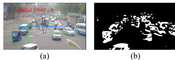
Figure 03: (a) Sample frame for detection and counting vehicle (b) Grayscale image of the sample frame
