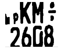
Figure 4. Eroded Image of Plate
